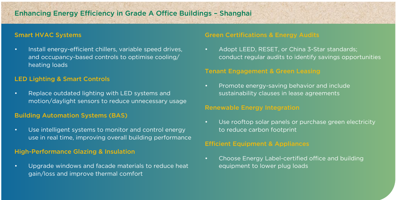
Figure 10: Select ways a typical Grade A office building in Shanghai can become more energy efficient
